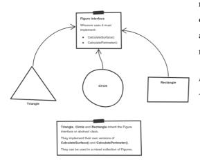
For example, in the figure above, the structure of the classes triangle, circle, and rectangle is inherited from the interface Figure, but the implementation of the methods will not be the same and would be overwritten.
