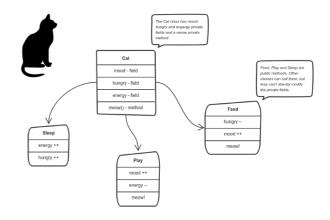
In the figure above, all the attributes and methods are encapsulated in each class.
